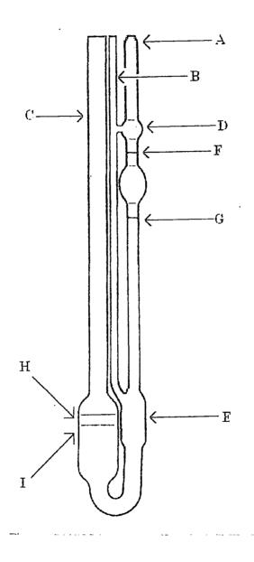
Figure 1. Ubbelohde Viscometer
