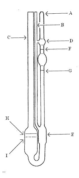
Figure 1. Ubbelohde Viscometer
